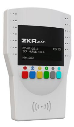
You can have detailed information and log reports on each interaction made with the built-in Mifare Card Reader on the Room Control Unit.
