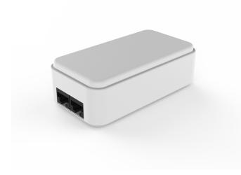
Provides control of On/Off for two different functions within the room (such as reading lamp or window blinds) from the patient handset. One Function Control Module must be installed per one Patient Handset, connected between the Room Control Unit and the Bedside Call Unit via its two RJ45 ports (in/ out).
